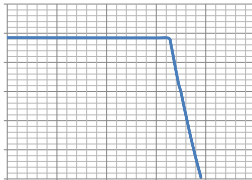
Figure 2. 4.85V LDO Vout vs Iout @Vin=6V
