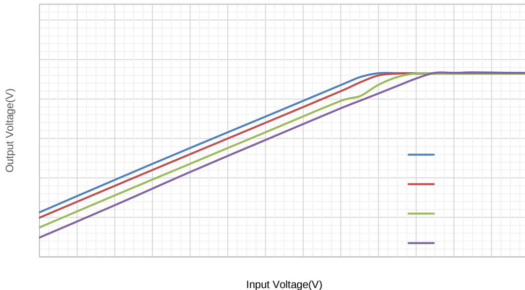
Figure 10. LDO Operation Characteristic ( V_{OUT}=5V )
