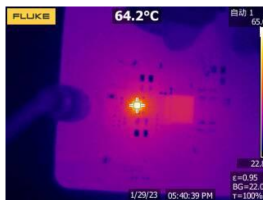
Figure 23. Thermal, 12VIN, 5VOUT, 3.5A
